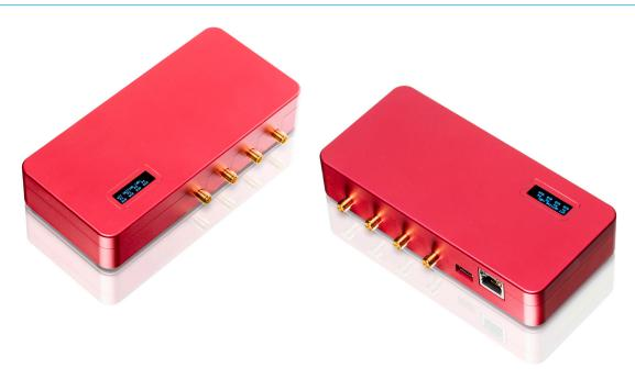
The MWave four-port attenuator is ideally suited to testing multi path communications channels (eg G.hn) under a wide range of attenuation levels, allowing different cable loss scenarios to be emulated.
